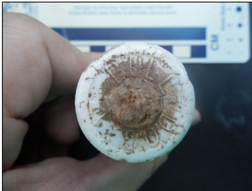
Figure 4.24: Bulldog Insulator, Illinois Electric Porcelain Co. of Dry-process Porcelain Dating Between 1910 to 1919
