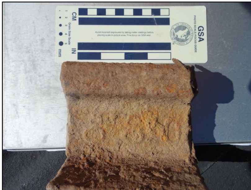
Figure 4.19: Tram Road Rail, Note Embossed Numbers
