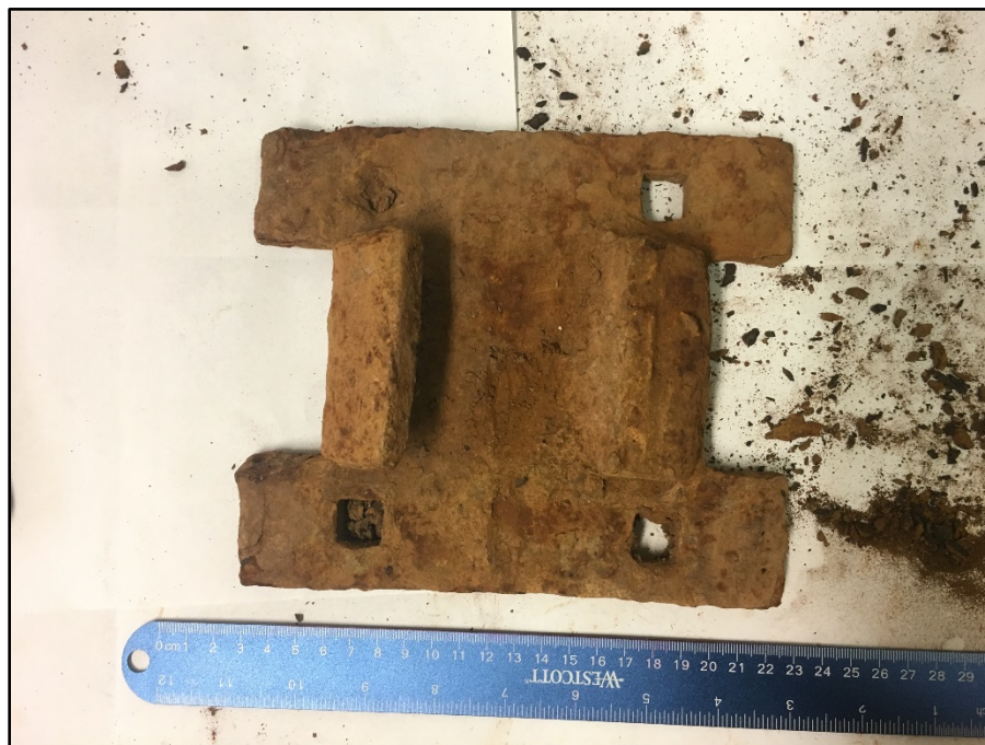
41FB355-21 Tie plate from moveable sugarcane tram track
